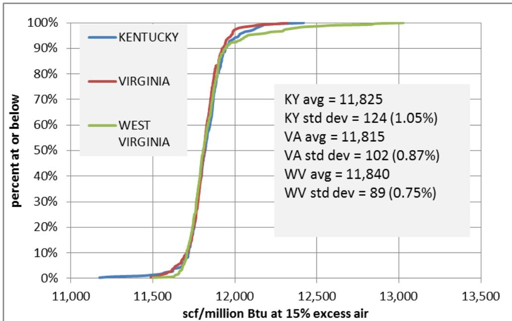
**Figure 4d.** Cumulative probability of lbmol CO<sub>2</sub> to heat input for Central Appalachian coal
