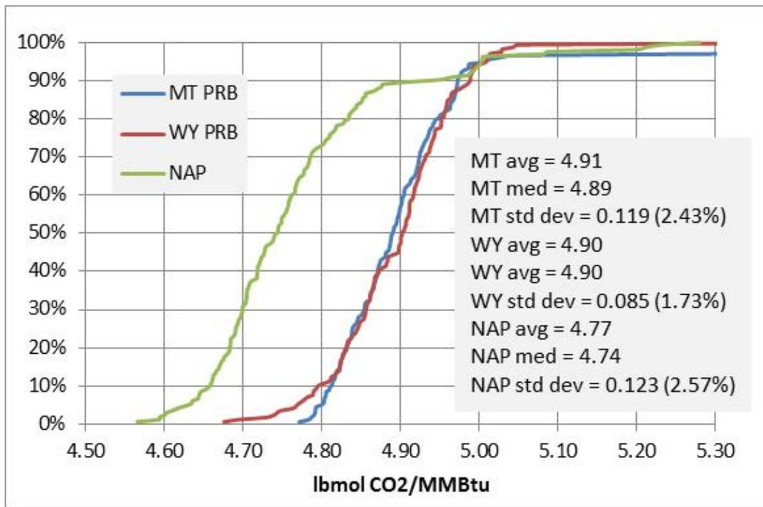
**Figure 4c:** Cumulative probability of exhaust flow to heat input at 15% excess air for Kentucky, Virginia and West Virginia Central Appalachian coals
