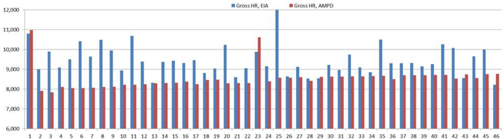
2014 Gross Heat Rate, EIA versus AMPD heat input (developed from EIA 923 and AMPD)
