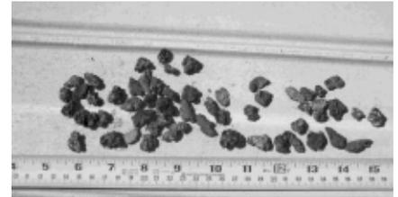
**4. Popcorn ash.** These photos of typical popcorn ash particles from a U.S. coal-fired power plant are of significant size (up to 1 in.) and specific gravity (between 0.2 and >1). *Courtesy: Southern Company*
