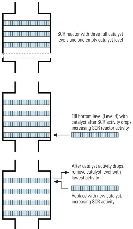
point, the regenerated catalyst is then added to the empty catalyst level, and the catalyst level with the lowest activity is then removed for regeneration.
