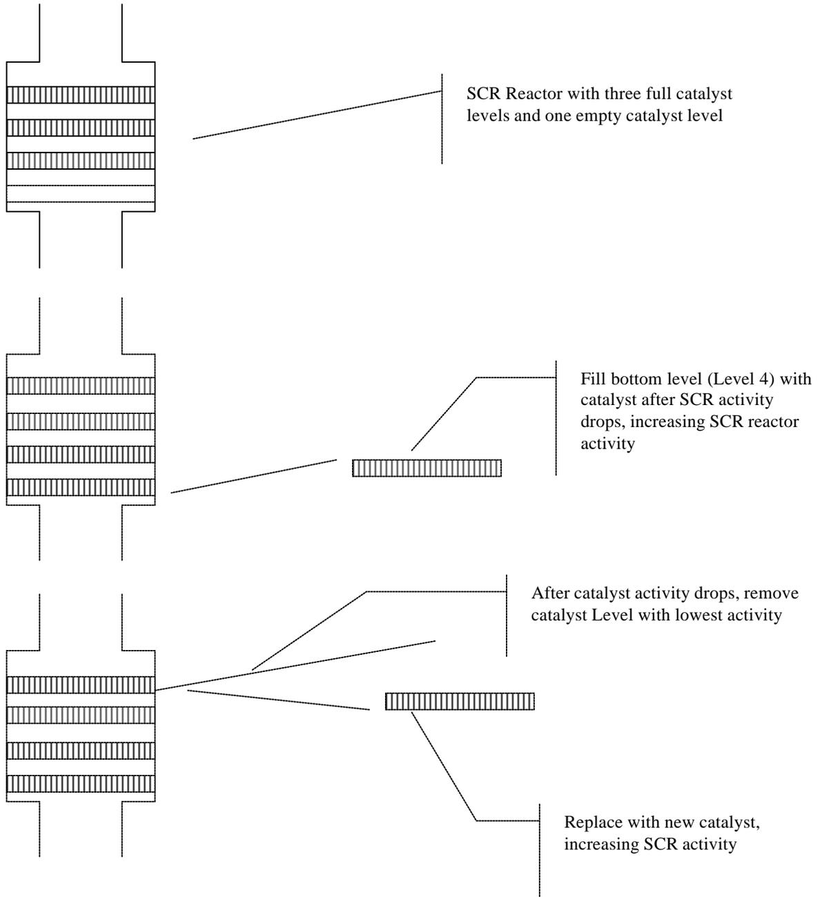
After the SCR reactor is full, it is necessary to replace catalyst levels with new or regenerated catalyst to increase total SCR catalyst reactor activity. This is shown at the bottom of Figure 1. Since the top level usually loses activity faster than the others, it is normally the first catalyst level to be replaced.
