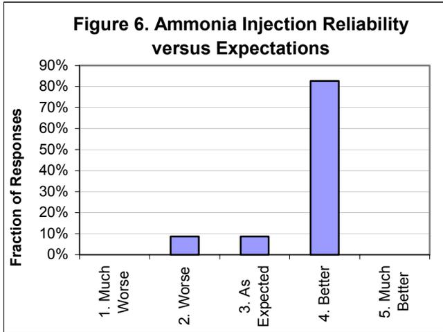
Figure 6 shows the distribution of responses regarding ammonia injection equipment. Fortunately, most respondents found this equipment to meet or exceed expectations. Furthermore, in the small number of cases where reliability of ammonia injection equipment was worse than expected, the problems were short term and correctable. So, these problems should not adversely affect reliability in the long term.
